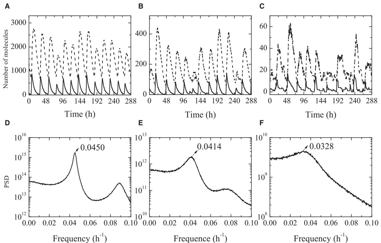
FIGURE 6 Robustness of circadian oscillations to molecular noise. (A–C) Oscillations of the amounts of *frq* mRNA (solid lines) and FRQ (dashed lines) with different  $\Omega$ : 100 (A), 10 (B), and 1 (C). (D–F) The power spectrum density (PSD) of FRQ amount corresponding to the above panels. The peak frequency is marked in the panels, and the corresponding period is 22.22 h (D), 24.15 h (E), and 30.49 h (F), respectively.
