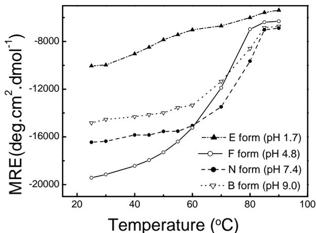
Fig. 4. Thermal denaturation of BSA monitored by far-UV CD at 222 nm for different isomerization forms.
