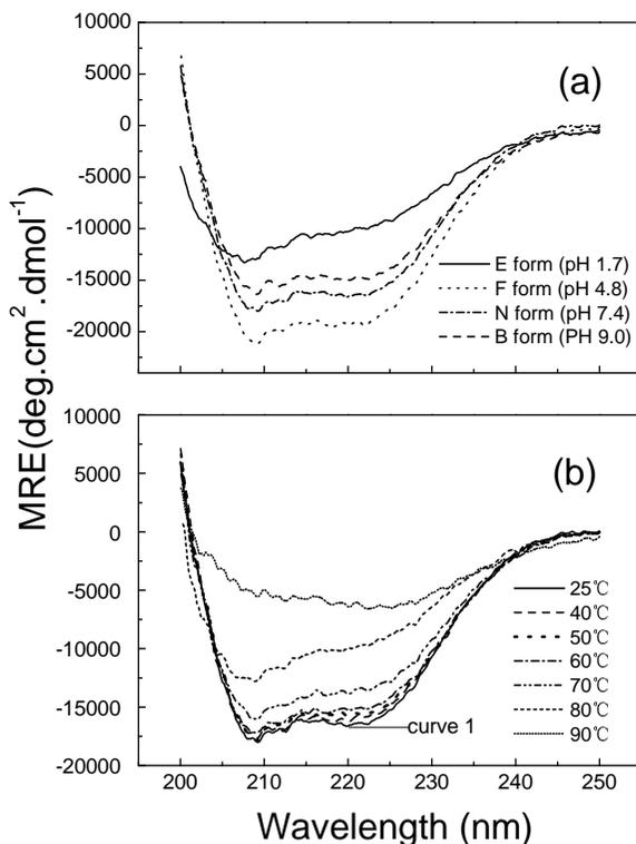
Fig. 3. Far UV CD spectra for different isomerization forms of (a) BSA and (b) thermal denaturation of native BSA in the N-form (0.2  $\mu$ M) from 25°C to 90°C.
