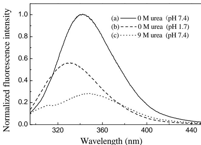
Fig. 1. Fluorescence emission spectra of 2  $\mu$ M BSA after excitation at 280 nm. (a) Native state; (b) acid-induced isomerization form; (c) urea-induced unfolded state.
