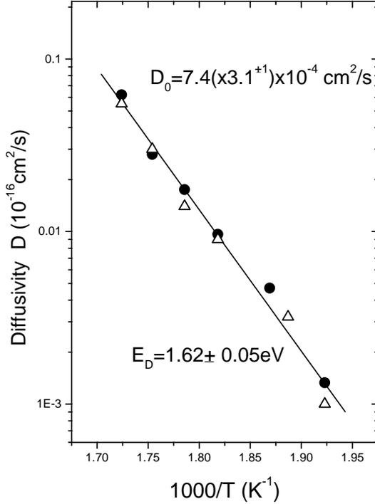
Fig. 5. Temperature dependence of the diffusivity  $D$  of  $\text{Ir}_{18}$  cluster migration on  $\text{Ir}(111)$  obtained from the mean-square displacements. The solid circles are our simulation results and the open triangles are experimental results cited from Ref. 15.
