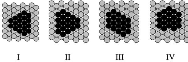
Fig. 1. Four nonequivalent forms of Ir<sub>18</sub> cluster on Ir(111). There are one configuration for each form I and form II, and six equivalent configurations for each form III and form IV. But only one configuration is shown for each form (see Ref. 12) All these fourteen configurations have a same total number of nearest neighbor atoms, 78, and are the energetical equilibrium positions for the atoms in the cluster.
