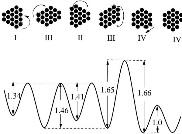
Fig. 3. Jumpings of the “dimers” between different forms. A couple of atoms with dashed line circled is the dimer which jumps from one energetical position to another. The movement is indicated by the arrow which shows the overall changes of the dimers. The effective energy barriers  $E_{\text{eff}}$  of several dimer jumping processes are marked. The exact values for the barriers come from the best fitting of the diffusivity with the experimental results in Fig. 5.
