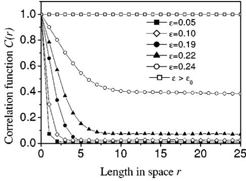
FIG. 5. Relationship between the spatial correlation function and the length in space in the case of  $\mu=3.4, L=500$  for different coupling strengths  $\epsilon=0.05, 0.10, 0.19, 0.22, 0.24, > \epsilon_0$ . The critical value  $\epsilon_0$  is 0.28.
