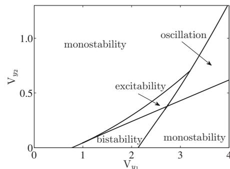
FIG. 10. Two-parameter bifurcation diagram in the space spanned by  $V_{y_1}$  and  $V_{y_2}$  with  $S=1$ . The dynamics of the system are mainly classified into four regimes: monostability, bistability, excitability, and oscillation.
