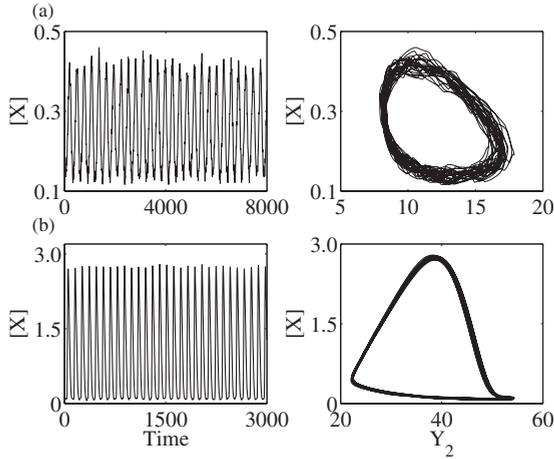
FIG. 8. The dynamics of the system in response to a noisy stimulus. The left columns show the time course of  $[X]$ , while the right ones show the corresponding phase plots of  $[X]$  vs  $Y_2$ . The strength of positive feedback is  $V_{y_1}=0$  (a) or  $V_{y_1}=1.5$  (b), while the strength of negative feedback is  $V_{y_2}=2$  and the time delay is  $\tau=50$  for both cases. The noisy stimulus is a series of uniformly distributed pseudorandom numbers between 0.5 and 1.5.
